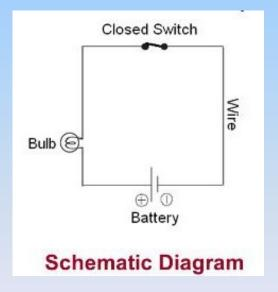
Note that the switch needs to be closed in order to let the current flow in the circuit and the lightbulb glow. When the switch is open, however, there is no closed path through which electrons can flow, therefore no electric current.
