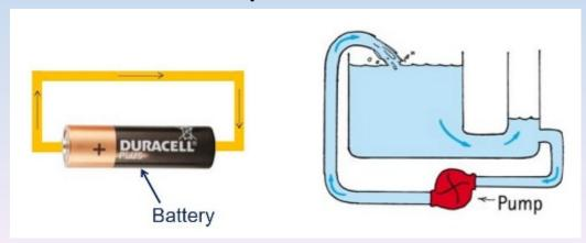
A battery uses chemical reactions to produce a difference in electric potential between its two ends, or terminals.
