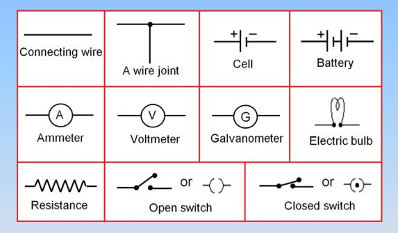
A **voltmeter** is an instrument used for measuring electrical potential difference between two points in an electric circuit.
