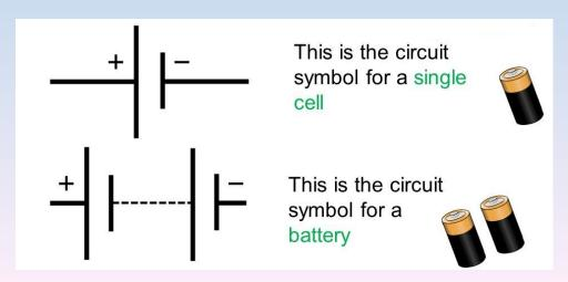
The terminal corresponding to a high electric potential is denoted by a + and the terminal corresponding to a low electric potential is denoted by a - .
