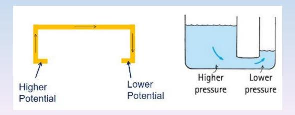
To maintain a continuing flow of water in the pipe, a pump must be provided to maintain the pressure difference.
